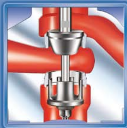
Variable: diverting plug
